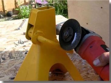
Use the Angle Grinder with the Zip Disk to cut off the remainder.
