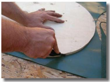
Place your Plywood circle on the Rubber Mat and using your Craft Knife carefully cut around the edges.
