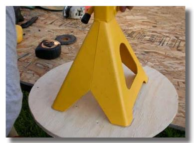
Align the Jack Stand onto the Plywood, lining up your corners with the marks you made previously.
