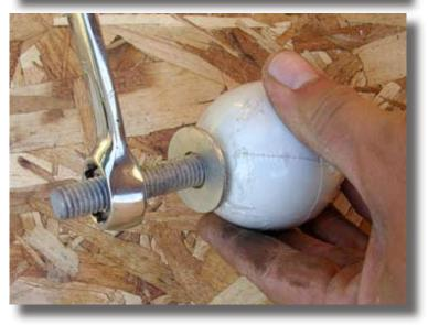
Insert the Bolt through the hole you just drilled. Place the Washer on the Bolt and then the Nut and tighten.
