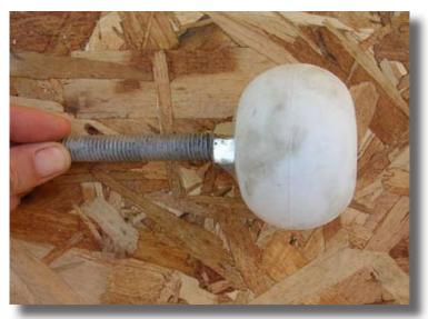
Tighten the Nut until the top of the Bolt is pulled into the Ball, squashing the ball slightly (see photo below for finished product).
