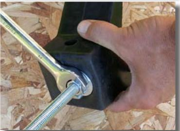
Tighten the Nut until the top of the Bolt is pulled into the Bow and is flush (see photo below for finished product).
