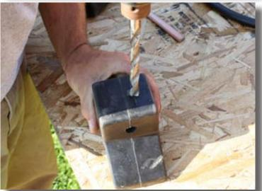
Using the large drill bit (size to match your 6" Bolt), drill a hole where your two lines cross.
