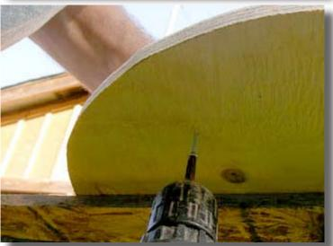
Using the Drill and the Phillips Head Drill Bit, screw the Self-taping Screws into the Plywood (using the pilot holes you made at each corner) and though the metal triangle plates on each corner of the Jack Stand. You need to be very accurate for this step and it's useful to have someone else help you hold the stand whilst you drill.
