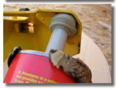
Apply a large blob of PL Glue onto the bottom of each leg of the Jack Stand.
