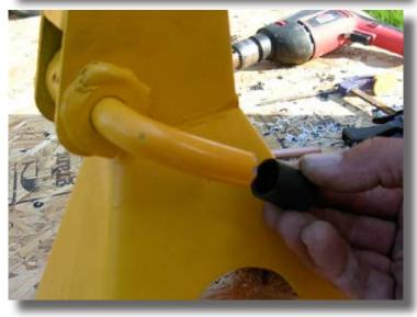
Replace the rubber cap on the handle.
