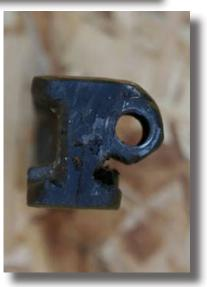
Once the weld has cooled, paint Rest, Nut and joint with black spray paint.
