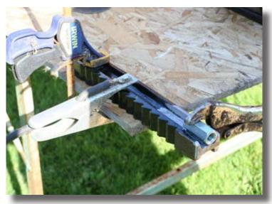
Clamp the Rest onto a stable surface and position the 2" Nut so that it aligns with the top (cut) edge of the Rest.
