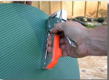
Use the Staple Gun to attached the Rubber to the underside of the Stand.
