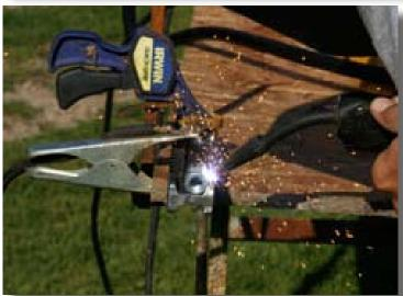
Weld the Nut solidly onto the Rest.
