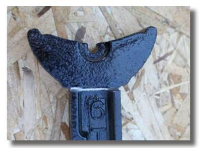
Take the Jack Rest and cut the top off using the Angle Grinder with the Cutting disk.
