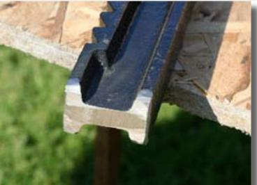
Remove paint on one side with the Angle Grinder and Zip Disk to provide a clear/ clean space to weld the 2" nut onto.
