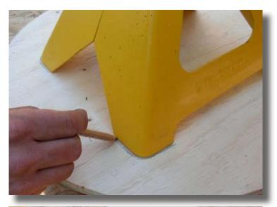
Place the Jack Stand in the center of the circle and mark around the four leg corners.
