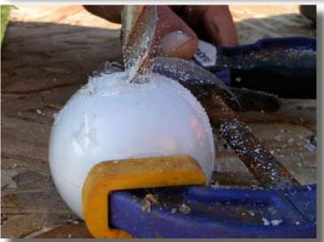
Use the Large Drill Bit to drill a hole through the center of the Ball.
