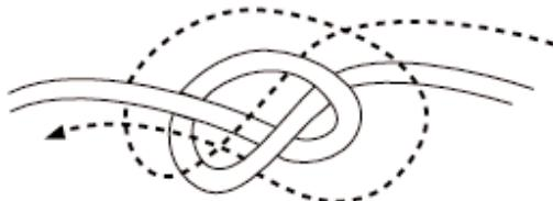
Tie into the left nose knot first. Then then right nose knot to make a double rope over the nose. (*Editor's note: remember to keep the rope laid out as shown...you'll regret it if you don't!*)
